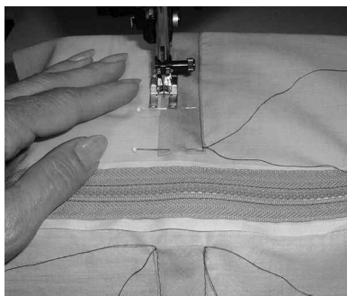
1) Edgestitch casing in place.
