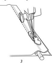
To finish an unfaced edge with piping, finish the piping/project seam allowance edges with zigzagging or serging to prevent raveling, then turn the seam allowances to the wrong side and topstitch close to the piping to hold in place. For a quicker finish, fuse the finished edges under using fusible web tape.
