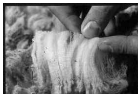
Fiber crimp makes for fuzzy wool fabrics.
