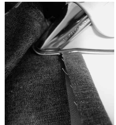
(3) Inserting fusible hem tape
